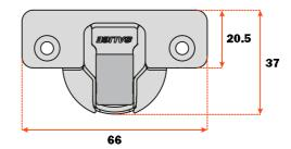
Constant "L" value of 1.3 mm (it does not change during side adjustment).
